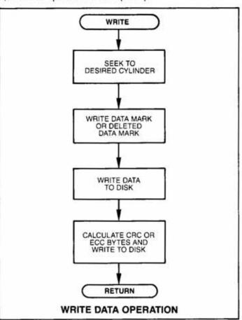
Before writing data to the selected disk drive, the UDC will read the current ID field, step to the desired cylinder (if enabled in command) and verify that has located the correct cylinder and sector. (These steps were described previously under "UDC Command Overview").
