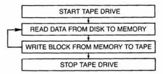
Control of a streaming tape drive is similar to that of a start/stop drive. The tape is started at the beginning of the data transfer and stopped after the last block is written to the tape. The tape is not stopped in between blocks. The UDC will however turn the Write Gate sig-
