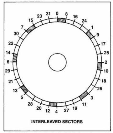
The UDC can format a track with interleaved sectors by staggering the sector numbers. For example, to format a 32 sector track, with a sector interleave factor of 4, the system processor would set up the ID Field table sector numbers as follows:
