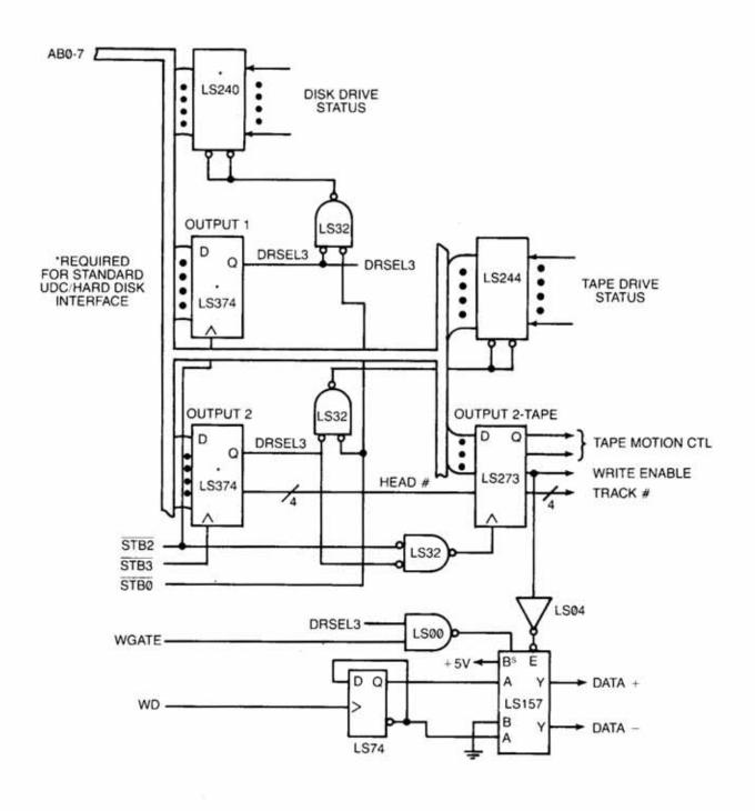
SCHEMATIC 2: HDC9234 TAPE DRIVE INTERFACE CIRCUIT
