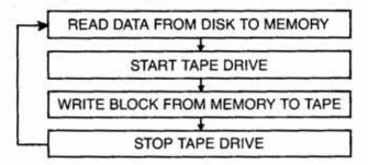
When controlling a start/stop tape drive, the UDC will write the data "block by block". The system will issue a Drive Select command to the UDC with the Tape Motion, Motor On and Write Enable bits set to start and write data to the tape.
