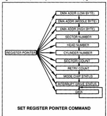
reduces the number of times the user must set the register pointer during read and write operation.
